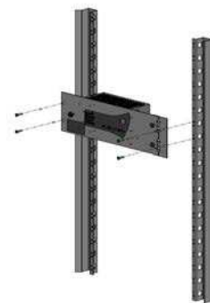
Rack F3U – Afm: 482x133x110mm – IP30
