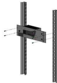
Rack F3U – Dim : 482x133x110mm – IP30
